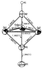
Figure 4. The bicapped tricobalt  $Co_3(NO)(NH)$  core of the  $[Co_3(\eta^5 - \eta^5 - \eta^5$  $C_5H_4Me)_3(\mu_3-NO)(\mu_3-NH)$  monocation (IIIb) with its independent interatomic distances under crystallographic  $C_1-1$  site symmetry. The position of the nitrene hydrogen atom was located from an electrondensity difference synthesis.
